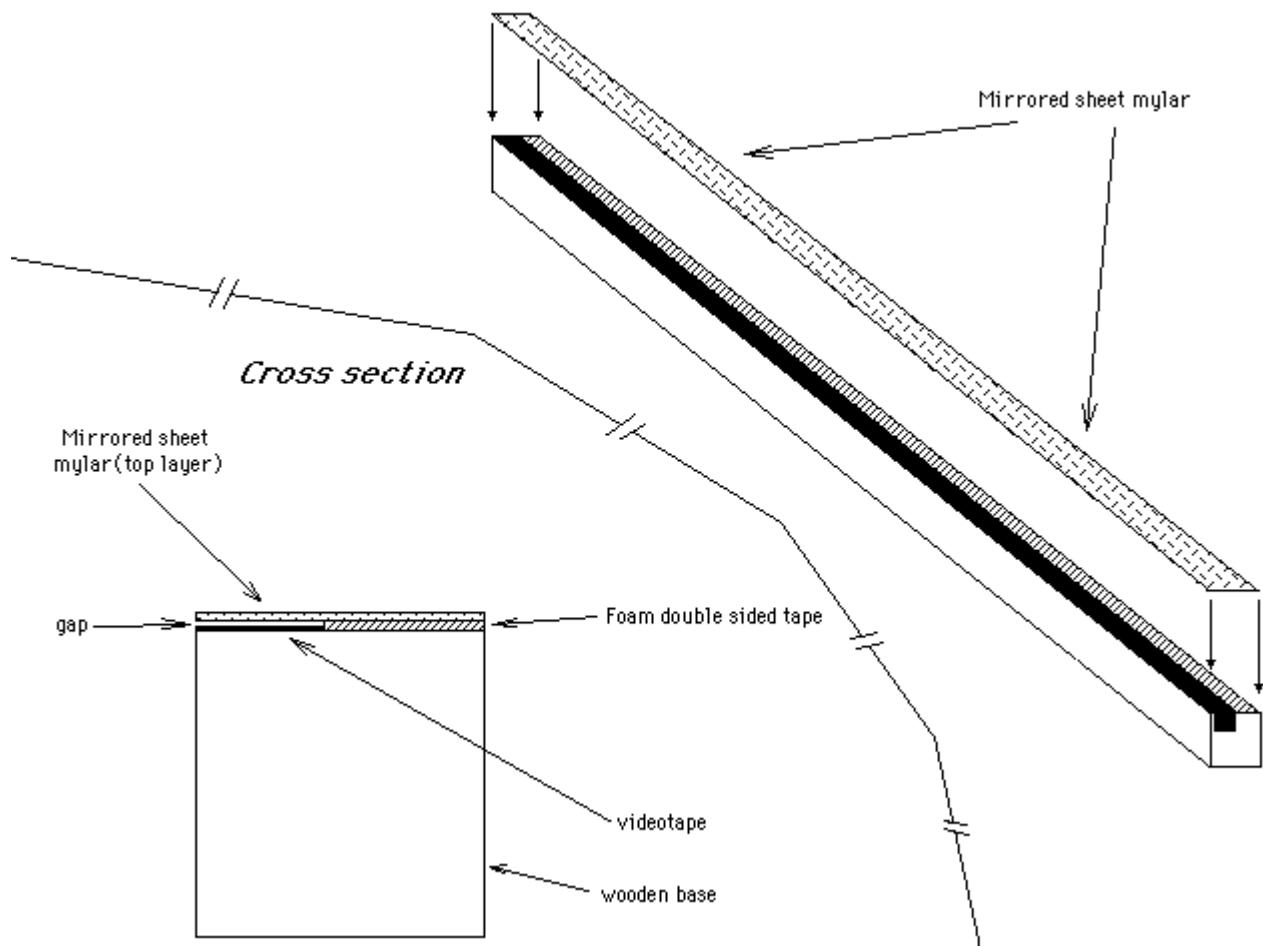
The trickiest part is making two good electrical contacts...one with the conductive videotape and one with the mirrored mylar sheet. I used small brass screws and washers, functioning as terminals. Careful to keep the videotape terminal(Point A) isolated from the mylar terminal(Point B).
